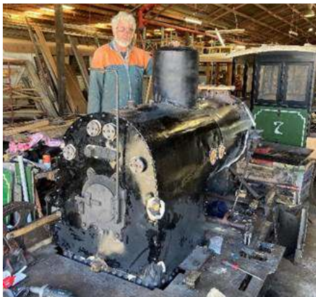
Reclad replacement boiler
